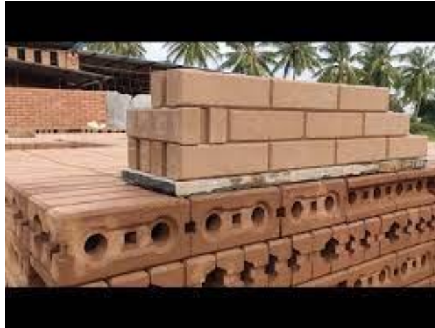
Figure 5: Above the red bricks are compressed earth blocks.
