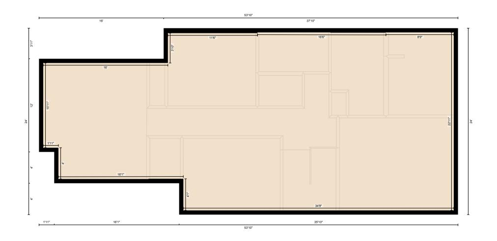
Measurement Diagram for: Basement Exterior Wall Thickness: 6.5 in
