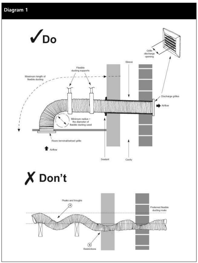
The inner radius of any bend should be greater or equal to the diameter of the ducting being used. If the radius is reduced, the resistance of the bend will increase and the volume of air being extracted will decrease (see "Do" Diagram). Ensure flexible ducting is installed without peaks or troughs (see "Don't" Diagram).
