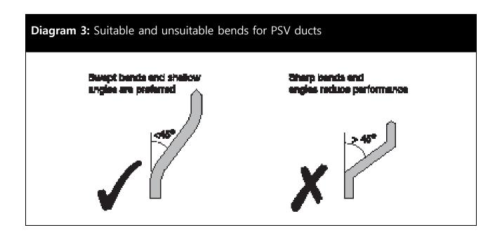
Ducts should use no more than one offset (i.e. no more than two bends) and these should be of the "swept" rather than "sharp" type to minimize flow resistance. Offsets at an angle should be no more than 45° to the vertical (Diagram 3).
