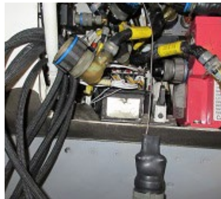
Right Main Line Power Contactor 1K-D008 Damaged
