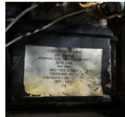
Right Main Line Power Contactor 1K-D008 Damaged
