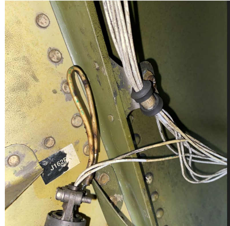
Discrepancy 32 – Extremely Severe cable bend could lead to premature conductor damage
