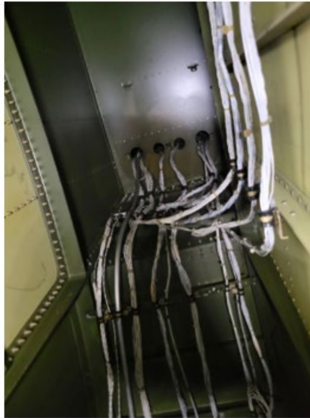
Figure 26 - Rubber Pass Through Grommets Missing (Discrepancy #23)
