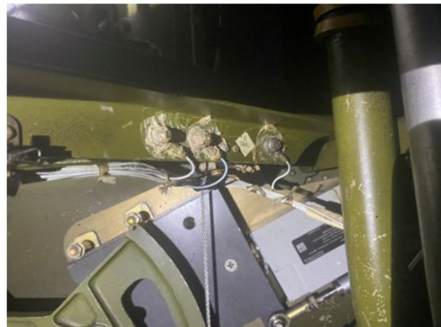
Figure 9 - E 5MU Grounding Terminals Bonding Adhesive Incorrect (Discrepancy #6)
