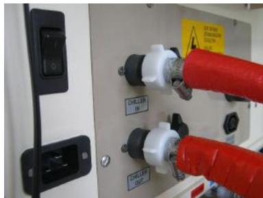
connect one hose to connection for „chiller out“
