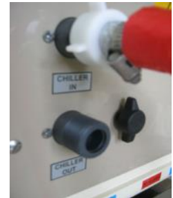
connect one hose to connection for „chiller in“
