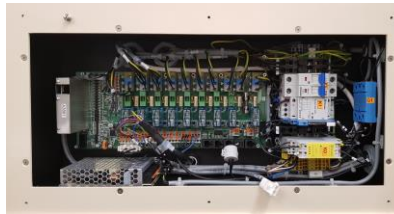
BE SURE THAT THE PROCESSOR IS DISCONNECTED FROM POWER SUPPLY! Open the electro box
