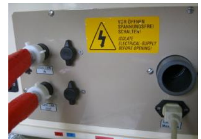
connect chiller cable to electrical connector „chiller“ of processor
