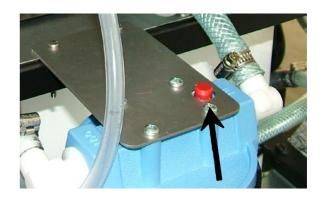
4. Fill in Cooling Liquid carefully up to 3/4 of the Filter using a funnel, while pressing the red button!
