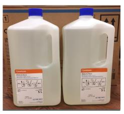
**STEP 2:** After mixing (2) 5L Bottles you now have (2) Empty 5L Bottles. Take the (2) 1L Bottles of Fixer Replenisher and pour them into the Empty 5L Bottles and Fill with Water. This Solution is now your Replenisher and is *to be used only to Replenish as needed*. Write an R on the Bottle with a Sharpie Marker to Identify this Solution as already mixed Replenisher and not Replenisher Concentrate.
