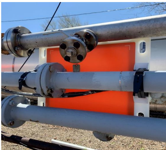
Mount kit with pipe cleats to reduce stress on the detector for pipeline imaging.
