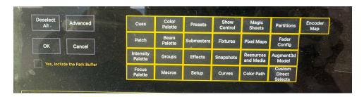
5. Under the "OK" button there is a checkbox that says "Yes, include the Park Buffer" It is very important to make sure this is checked or the board will not work.
