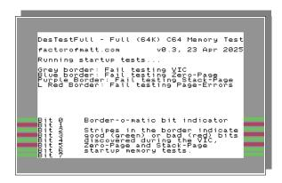
The border-stripes show data bits (D0-D7, top to bottom) that showed inconsistencies while testing the VIC-II registers. Here we see that data bits 1, 3 and 5 were detected as bad. This may be of diagnostic use if another data attached chip in the system is corrupting the bus – or it may simply indicate a marginal VIC-II.
