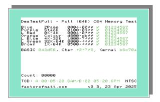
At the bottom of the screen is the count of the number of times we've looped through all the tests. Each cycle takes less than 30 seconds.
