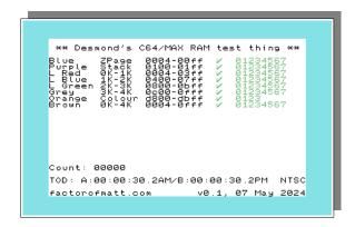
At the bottom of the screen is the count of the number of times we've looped through all the tests. Each cycle takes less than 30 seconds. The TOD information (derived from the CIAs if they're present) is mostly for decoration though may indicate CIA issues if the times look crappy.
