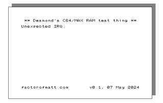
The receipt of an IRQ during the execution of tests could very well indicate something wrong with the interrupt-signal path or a misbehaving interrupt source (VIC-II, CIA etc).
