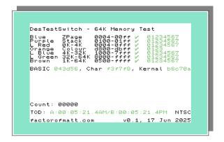
At the bottom of the screen is the count of the number of times we've looped through all the tests. Each cycle takes about 5 ½ minutes.
