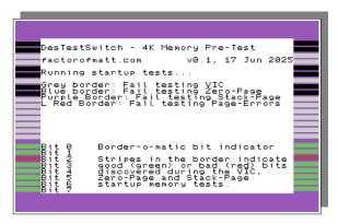
The border stripes show address bits (A0-A15, top-to-bottom) and data bits (D0-D7, top to bottom). A black address bit is 1, light grey is 0. A green data bit indicates a good bit, red indicates bad. Here we see that data bit 2 was detected as bad and that the most recent memory location found to be bad was \$01B3.
