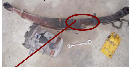
Lead spring and dryer part needed to repair bus.
