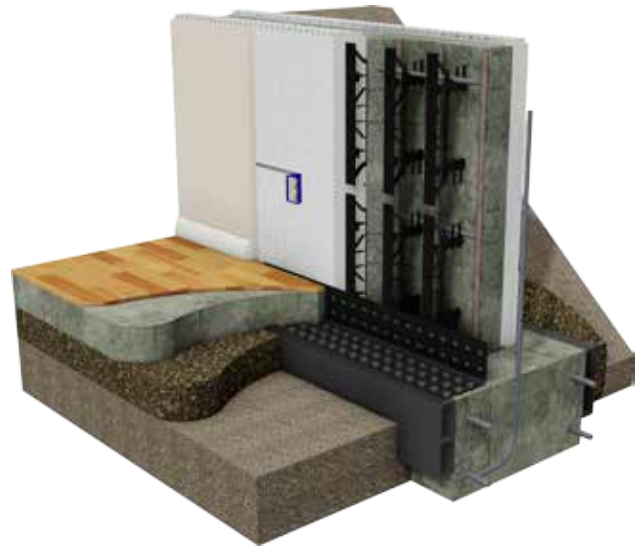
Figure 6.1.3 Basement wall showing footing using Form-A-Drain, and Cactus Board waterproof floor edging.
