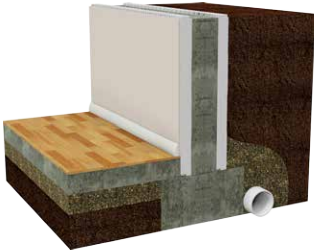
Figure 6.1.1 Standard poured footings with slotted PVC and gravel draining to daylight or a sump pump.
