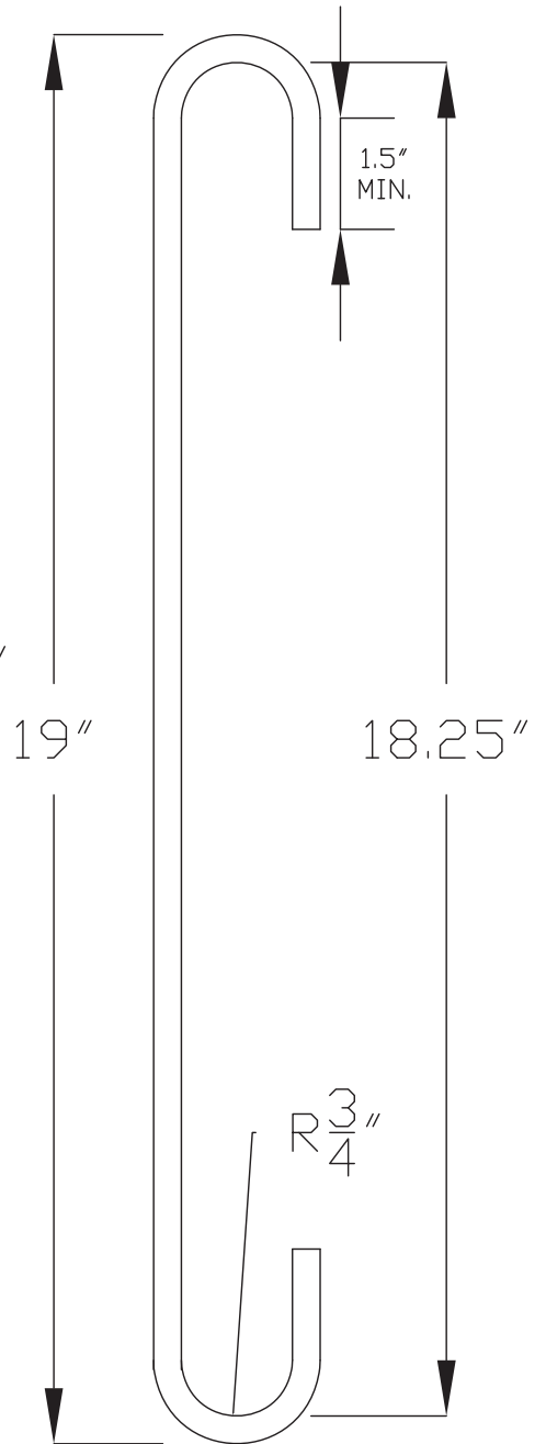
RECOMMENDED STIRRUP FOR BD-1200+8" RISER
