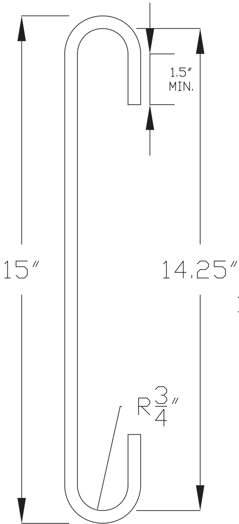
RECOMMENDED STIRRUP FOR BD-1200+4" RISER
