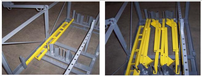
Insert the guardrails post 2 by 2 with the handrail and midrail members bracket on the same side.
