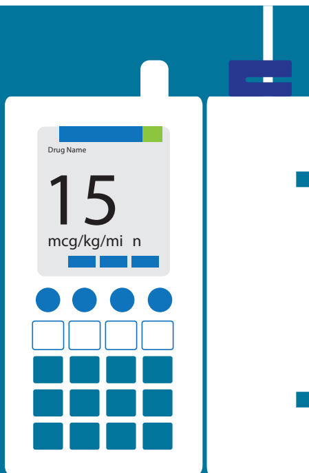
Figure 3. The SIGMA Spectrum Pump's Titration Error Prevention Feature alerts clinicians to dose increases or decreases exceeding defined limits, which can help identify potential medication titration errors.
