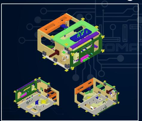
Designed and machined to precisely identify leakages in the component. It is composed of high quality rubber seals and interlocking mechanisms to hold component properly in place for inspection and monitoring of system that contains liquids, gases, or other substances to ensure that the contained materials do not escape, leak, or otherwise leave the system.
