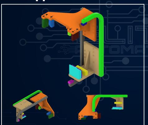
Designed to extract die cast component from die cast mold.
