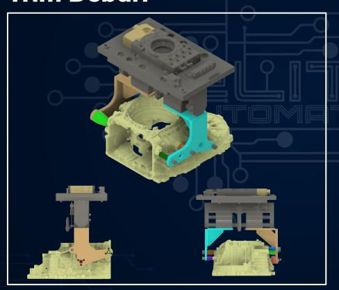
Designed to grip component for deburring process.
