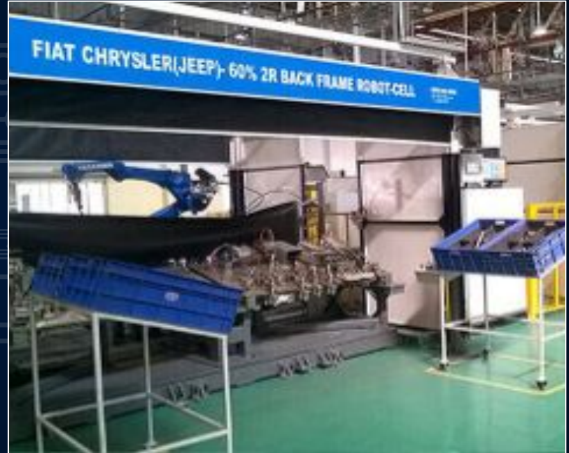
Arc Welding Cell With Positioner
