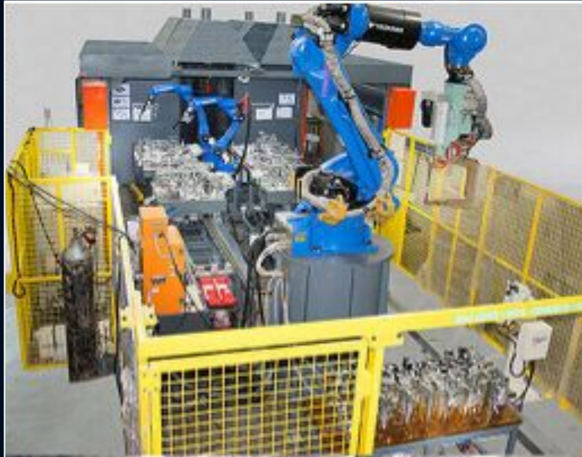
Spot & Arc Welding Cell
