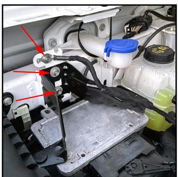
Remove the three (3) 8mm bolts as shown (the top bolt holds secures the vehicle computer ground wire to the vehicle while the bottom two bolts secure the computer bracket to the vehicle). Once these bolts are removed lift up on the factory mount and slide it out. You
