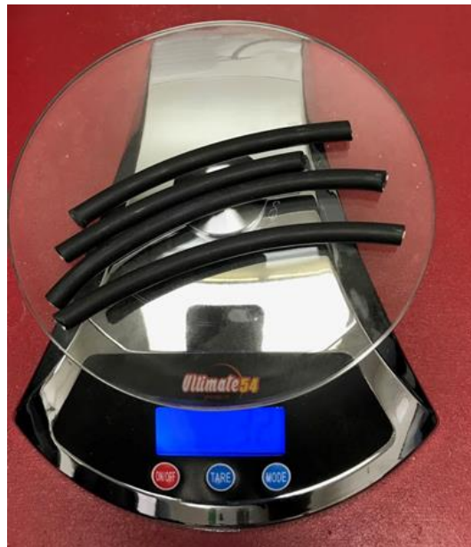
Figure 16 Cables removed from J-box to be weighed
