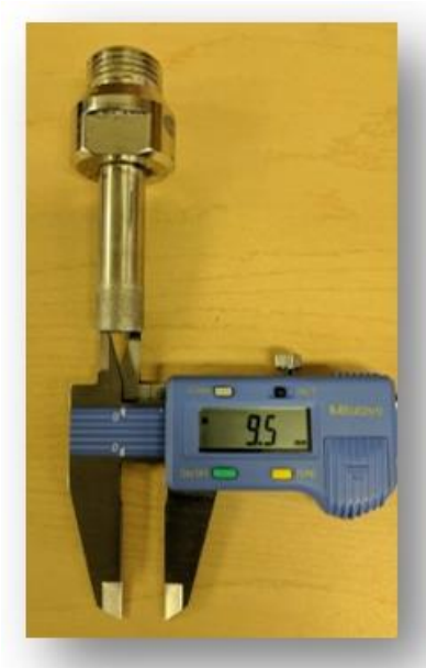
Figure 11 Diamond Coring bit used for extracting samples
