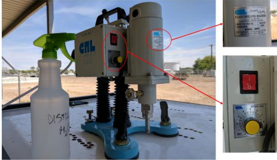
Figure 18 CRL Glass coring machine with diamond coring bit
