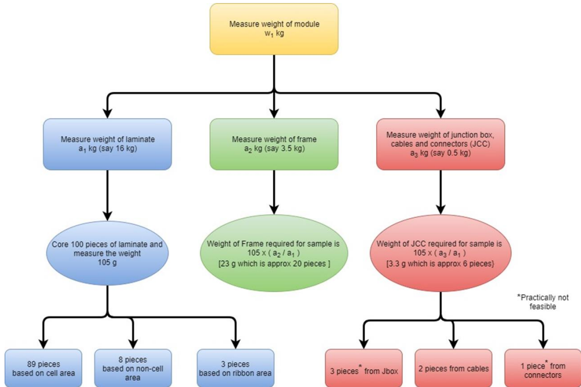
Figure 7 Ideal case approach for sample extraction
