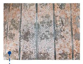
The customer's existing 1/2" woven screens were regularly blinding and plugged with material, requiring multiple shut downs in order to clean the screens to help minimize lost production and keep material in spec.
