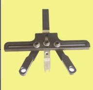
**BMW119-340 Chain Tensioner** To tension the primary timing chain on BMW N40, N42, N45, N46, N51, N52, N53, N54, N55, engines when setting valve, cam or VANOS timing
