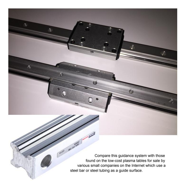
As might be expected, the cost of the above linear rails and roller cassettes is the most expensive part of the physical table. However, by limiting the size of the system and eliminating the manufacturer profit margin, you can complete your build for the same or possibly less cash outlay than a cheap ready-made unit.
