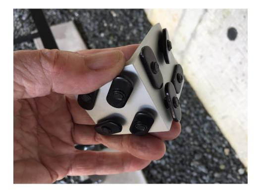
At each corner of the table, attach the 8 hole angle brackets as shown below.
