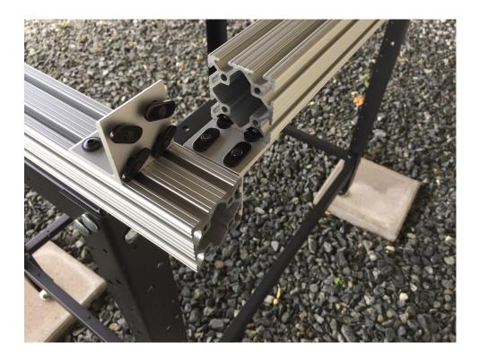
Note that by pre-assembling all the brackets, the 36" extrusions can simply be slid into place.
