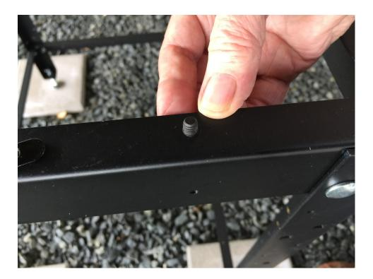
Screw one of the 1/4-20 T-nuts partially onto each button head cap screw, leaving about 1/4" gap underneath.
