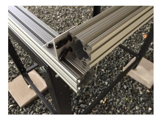
Tighten down all the button head cap screws, allowing the 36" extrusions to slightly overlap the 24" extrusions, as shown below.
