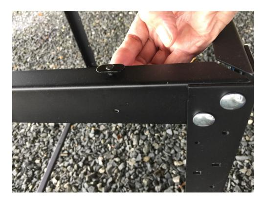
Slide one of the 30 1/2" extrusions onto each of the T-nuts on the end of the table.
