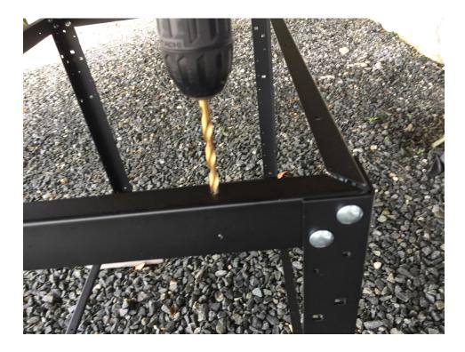
In each of the newly enlarged 1/4" holes, insert one of the  $1/4-20 \times 1/2$ " button head socket cap screws up from the bottom.
