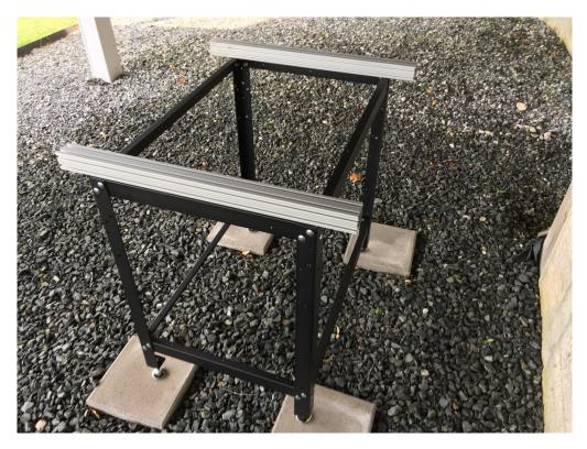
Using the  $1/4-20 \ge 1/2$ " button head cap screws and T-nuts, attach an 8 hole angle bracket to the inside end of each extrusion as shown. Below. The edge of each bracket should be about 1/8" in from the end of the extrusion.
