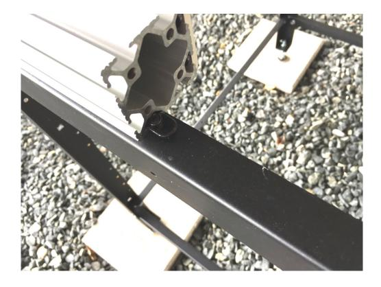
When you have finished attaching the extrusions to both ends of the support table, it will look like this.
