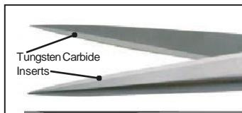
**Tungsten Carbide (TC) Scissors are manufactured with Tungsten Carbide Inserts in the blades of the Scissot.** Tungsten Carbide is much harder and longer lasting than Stainless Steel and is designed to provide a longer lasting sharp edge on the Scissor blade for many years. **Tungsten Carbide Scissors are designated by Gold Ring Handles.**
