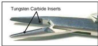
**Tungsten Carbide (TC) Needle Holders are manufactured with Tungsten Carbide Inserts in the jaws of the Needle Holder.** Tungsten Carbide is much harder and longer lasting than Stainless Steel and provides sharper teeth which are designed to provide a more precise and secure grip on the needles.
