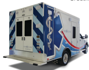
The all aluminum underbody bumper protects the module in low impact collisions.
