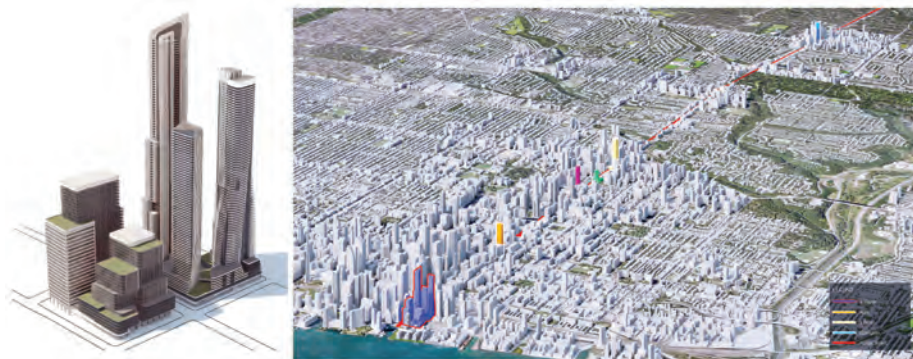
Figure 11. (left) Axonometric massing study highlighting terracing and balcony scheme; (right) tower height relationship study along the Yonge Street intensification corridor (Source: Hariri Pontarini Architects, 2016) 图11. 体量研究阐释梯次平台的设计方案轴测图 (左) 沿央街集约化地段高层建筑高度相关性研究 (右) (来源: Hariri Pontarini Architects 建筑设计所, 2016年)
