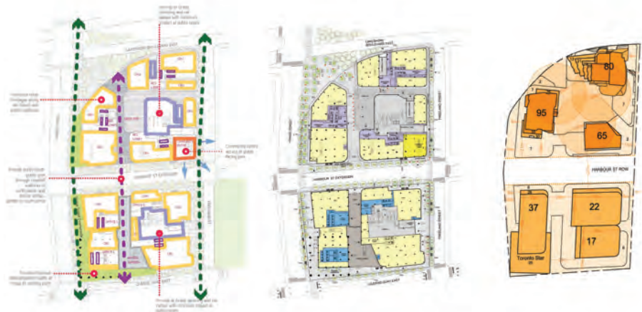
Figure 10. (left) Conceptual program and circulatory diagram, (center) architectural ground level plan, (right) height, separation, relationship, and terracing scheme, One Yonge (Source: Hariri Pontarini Architects, 2016)
