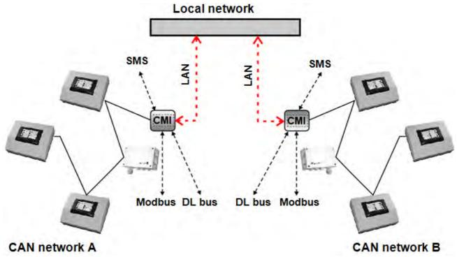
The **receiving** C.M.I. must have a **fixed** IP address. We recommend firstly installing the C.M.I. **with DHCP** and then **deactivating DHCP** mode in the Settings/Ethernet menu.
