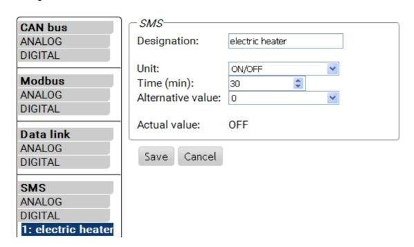
The SMS command *electric heater on!* sets the SMS input value **digital 1** with the designation "electric heater" to the value **ON**.
