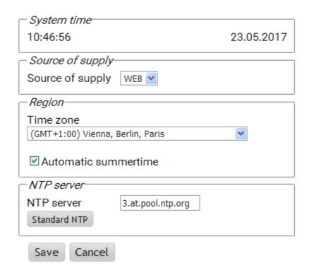
**Source of supply:** The C.M.I. accepts the time-stamp either from an adjustable NTP server (default setting: 3.at.pool.ntp.org) or from the CAN network (UVR1611 with node number 1) or via one of the two data lines (DL bus) of the respective connected controllers.
