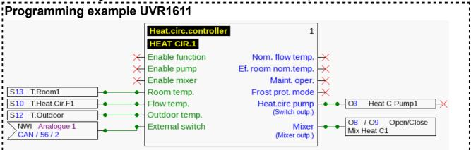
In the example above, the SMS input "**Heating**" was assigned to the CAN output **analogue 2** of the C.M.I. (node 56).
