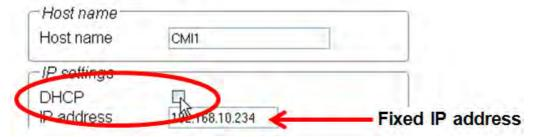
If data is transmitted in both directions, both C.M.I.s must have a fixed IP address.
