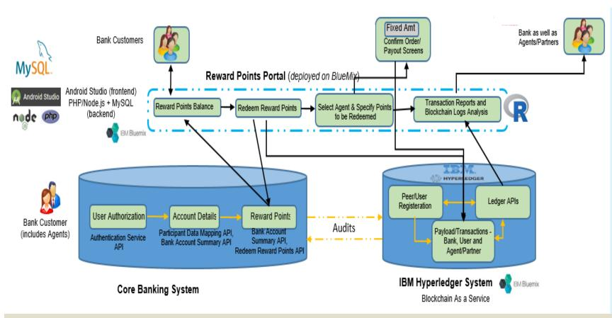
From an android app, customer authentication is managed through MySQL (stores client ID+Access Code) via a backend PHP running on Apache Webserver. If a correct match is found, the backend PHP generates an access token by calling up the Open Bank API from bluemix.
