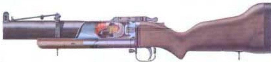
A single shot breach loading weapon that fired 40mm (1.57") Explosive Rounds or Buckshot rounds. The grenade round has a range of 400 meters (437 yards) while the buckshot was used at point blank range. The weapon weighed about 7lbs. loaded and was about 28 inches
