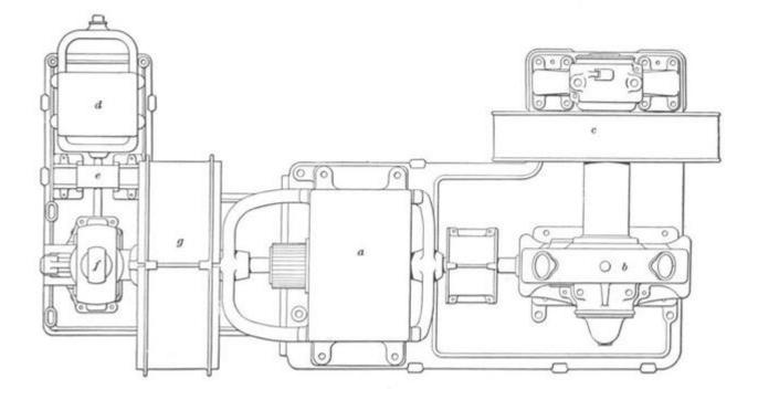
a- Is the main AC motor. b- No 1 size main gearbox c- Main traction sheaved- Micro drive motor e- Micro drive brake f- Micro gearbox Otis 1/4 machineg- Revolving brake that performs as a clutch, disconnecting the micro gearbox.
