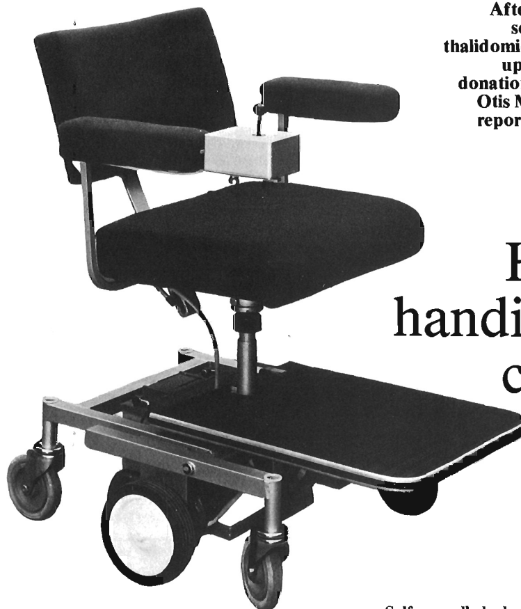
Self-propelled wheel chair made by Dennis Horner in Liverpool. It is controlled by the unit on the righthand arm rest
