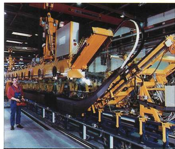
A balustrade assembly jig inside the completely re-equipped Otis escalator plant at Stadthagen.
