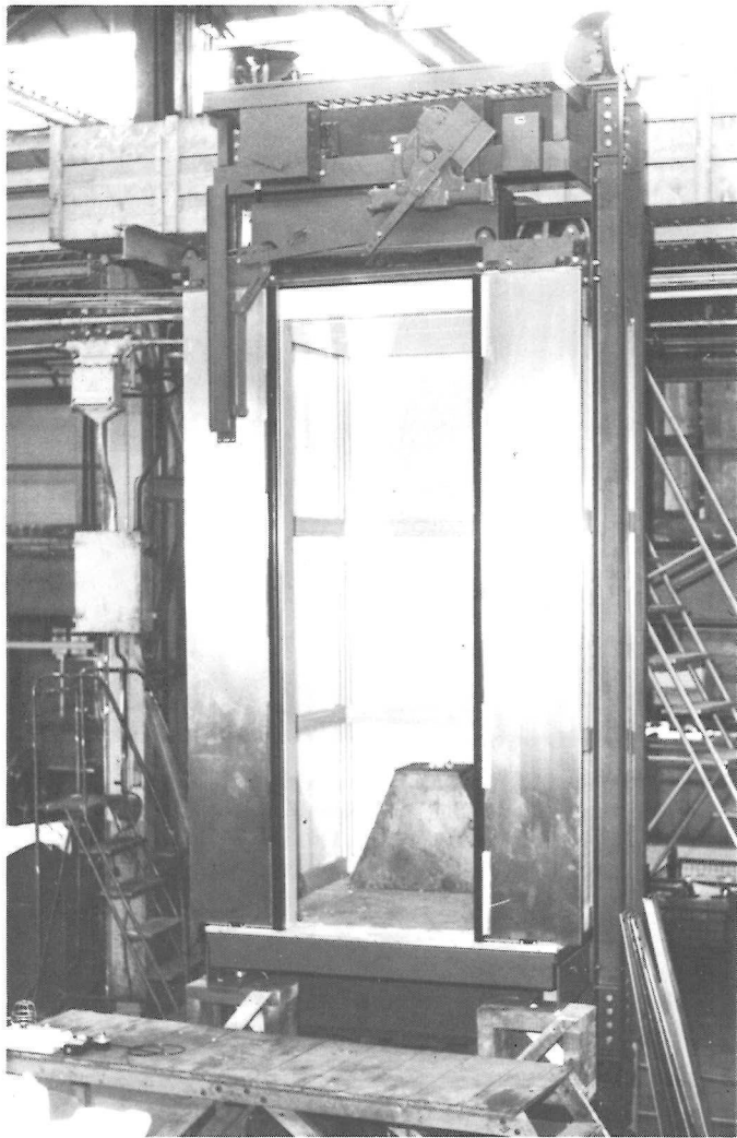
At Liverpool works the first glass-clad lift car stands ready for shipment to Hong Kong for the massive Hong Kong and Shanghai Bank contract which is being project-managed by UK's Ian Millar.
