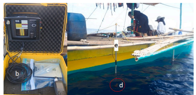
Fig. 3. Humminbird 698ci HD SI Combo primary components and set-up: (a) Main control head unit is connected via (b) 12-volt power cable to a (c) 12-volt power bank. The control head is also connected to a (d) small transducer that is side-mounted at/near the center-of-gravity of the outrigger boat with a (e) 1.8 m pole. (Notes: The safety rope from the transducer to the boat aids in stabilization of the transducer as it moves through the water during surveys. Whereas the control head unit is placed as near as possible to the transducer for more accurate, real-time measurements and recordings.)
