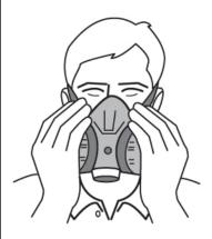
Positive fit check: With palms over exhalation valve openings, exhale gently into the mask. You should feel pressure in the facepiece.
