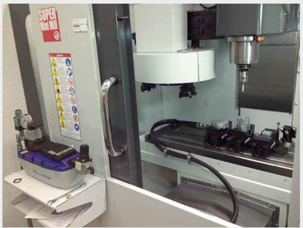
solinos 65-H 3 solinos 65-H angesteuert mit Pneumohydraulikaggregat solinos 65-H 3 solinos 65-H controlled with a pneumohydraulic unit
