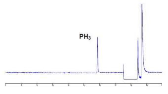
Figure 4. PH3 in Propylene at 1ppm
