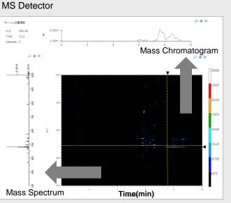
Figure 1 Contour Plot Based on DAD and MS Scan Analysis Results
