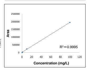
Figure 2 Calibration Curve Based on SIM Chromatograms
