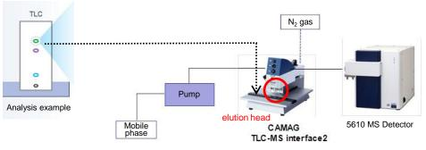
Figure 1 Example of TLC-MS System Configuration
