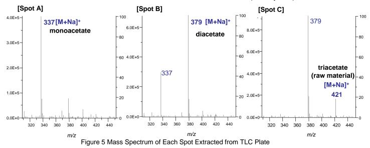
By directly extracting the target spot from the TLC plate and obtaining mass information, triacetate, diacetate, and monoacetate, for which identification was difficult due to insufficient separation only by TLC, could be easily identified. In many cases, there is no reference standard available for a product formed during the synthesis process and the mass information is useful for compound identification.
