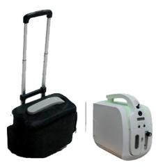
Technical Parameter: Oxygen Flow (L/min)1-5 Oxygen Purity (%)  $93\%\pm3\%$  ( 1LPM ) ,  $75\%\pm3\%$  ( 2LPM ) , $55\%\pm3\%$  ( 3LPM )  $45\%\pm3\%$  ( 4LPM ) , $38\%\pm3\%$  ( 5LPM ) Oxygen Pressure (Mpa) 0.03-0.07 Noise (dB)  $\leq$ 45 Dimension(mm) $350\times190\times320$  N.W. 6 kg. Rated Power (W) $\leq$ 75 Power Supply - AC220V
