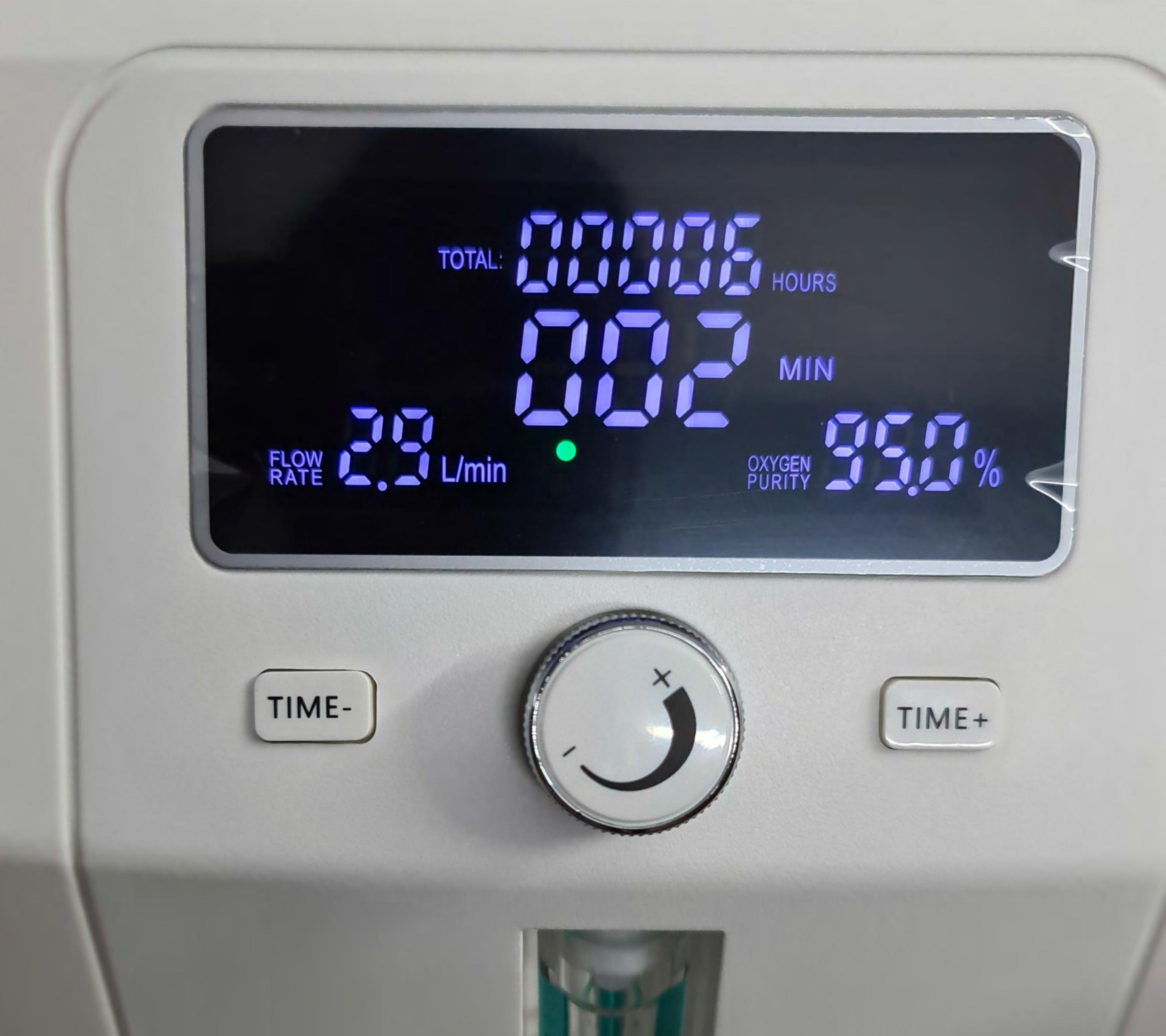
16. Main display indicating Hours & Minutes used, Digital Flow Rate, Oxygen Purity. You can use timer buttons to schedule timer. Adjust the knob to increase / decrease flowrate
