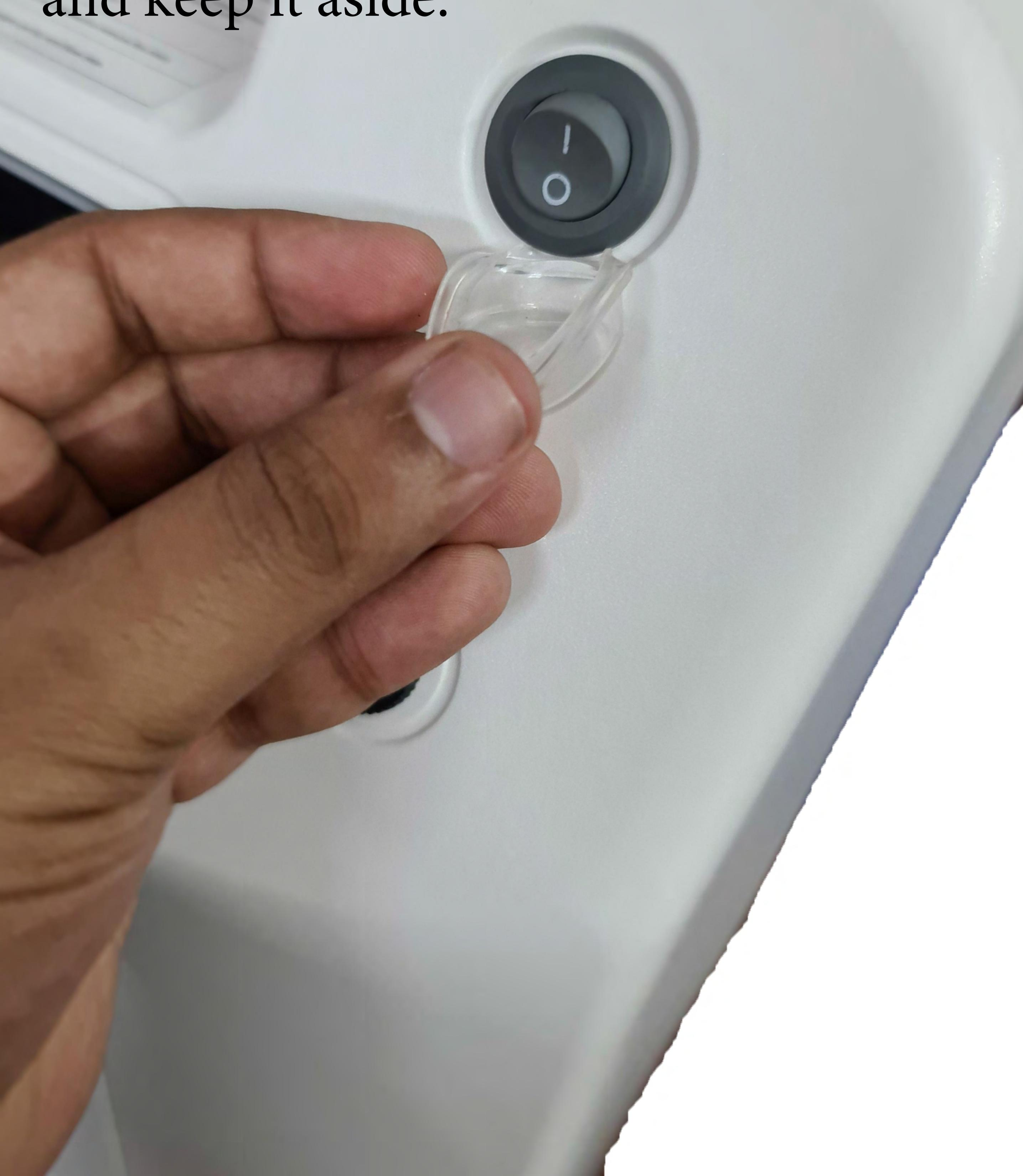
12. This step is very important, tilt the device and you will see two velcro straps. Unhook it and then only you should switch on. This is to protect the compressor during transport.
