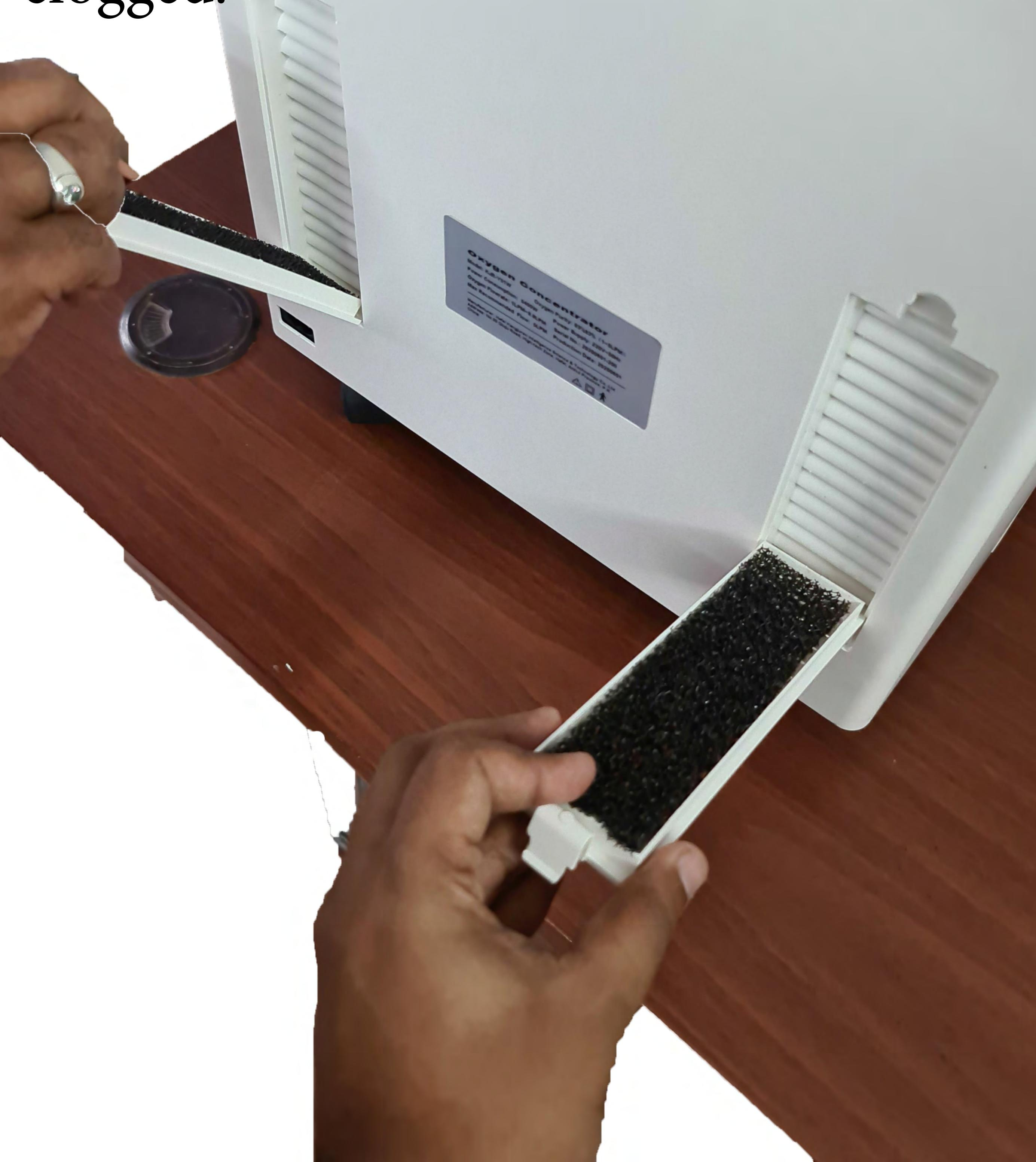
19. Remove secondary filter and dust it once in 2 weeks. Replace it when necessary and when it is fully clogged.
