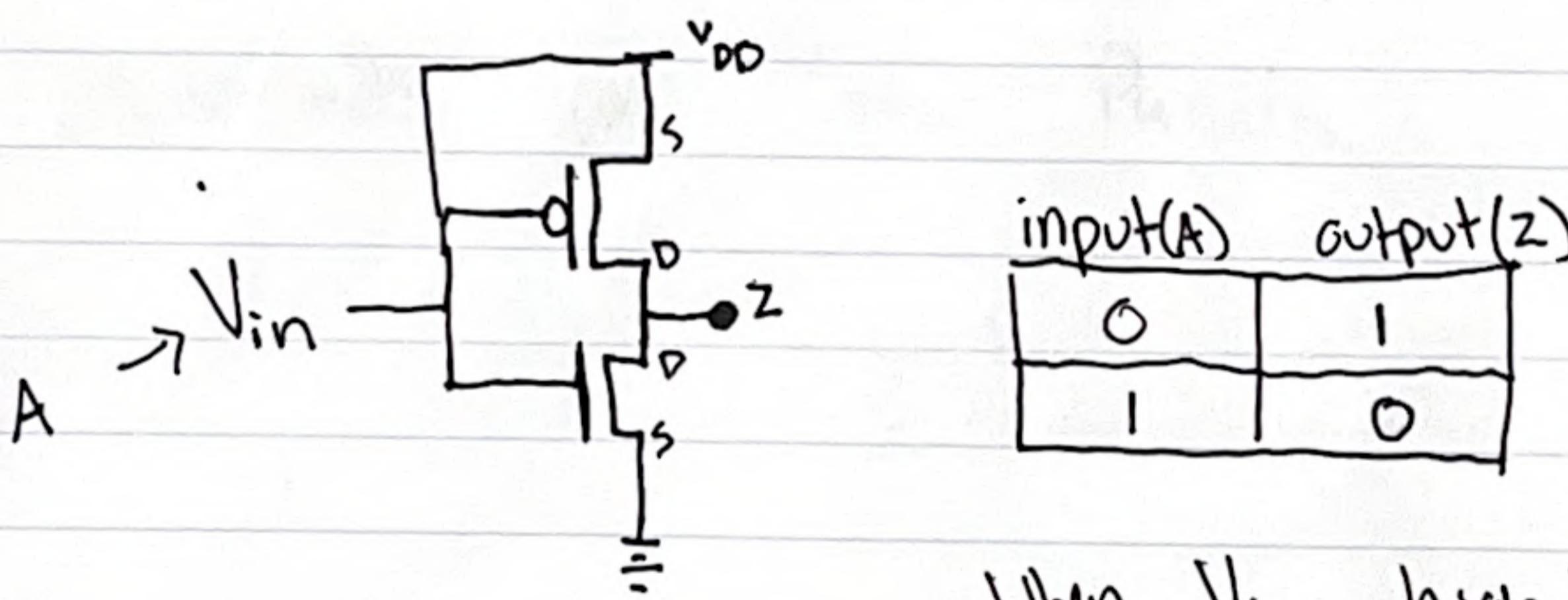
When  $V_{in}$  high: nMos ON
