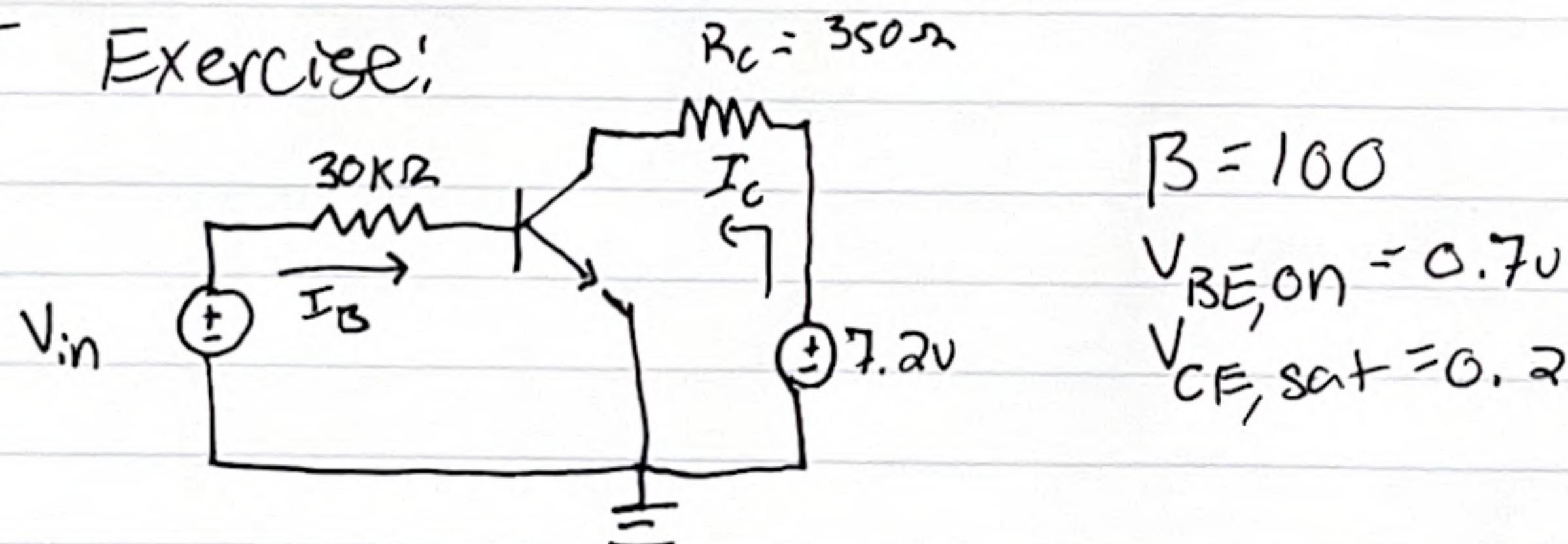
What  $V_{in}$  would cause the trans. to the edge of saturation
