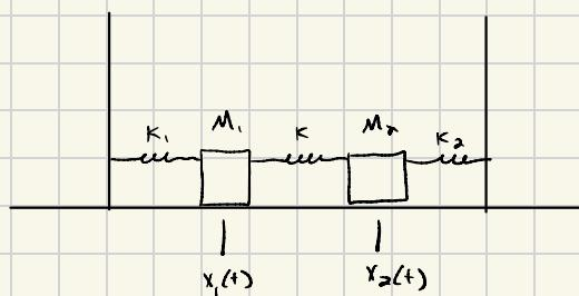
$$\left\{ \begin{array}{l} M_1 \ddot{x}_1 = -Kx_1 - Kx_2 + g_1(t) \\ M_2 \ddot{x}_2 = Kx_1 - Kx_2 - K_2 x_2 + g_2(t) \end{array} \right.$$
