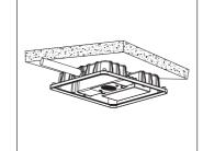
4. Disconnect the wires came from 3/4" hole and connect the wires came from 1/2" conduit with canopy . (White for Neutral, Black for Line, Green/Yellow Green for Ground)
