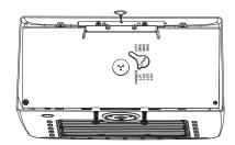
2. Knock off one of blind hole in the four sides of the mounting box to guide the wiring. Stick EVA gaskets on the back of the wall mounting box properly, which is very important for water proof. Fix the wall mounting box on the junction box according to the arrow pointing upwards.
