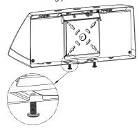
3. Hang the fixture on the wall mounting plate with a wire rope, and pay attention to protect the surface of the fixture during installation to prevent scratches and damage to the surface. Ensure the line voltage at the fixture is correct, make all necessary wiring connections, and push all the wires and wire nuts into the j-box.
