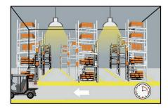
3 After elapse of hold time, the sensor dims the light at the present low light level if no motion is detected.
