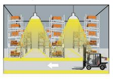
With insufficient ambient light, the sensor switches on the light when motion is detected.
