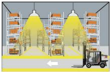
When motion is detected, the sensor will switch on the light to 100% brighteness
