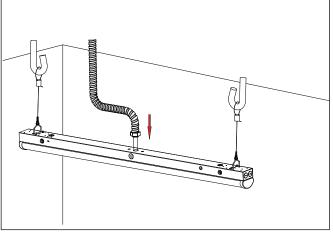
6. Insert the wire terminal joint to the wire entry.
