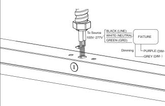
5. Insert the terminal block and wires into the strip.
